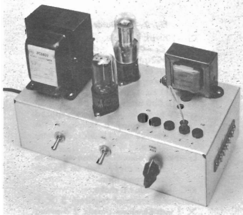
Fig. 4—The power-supply unit. Mounting of parts closely follows the circuit diagram of Fig. 6, with the power transformer at the left, rectifier (front) and voltage regulator tubes alongside it, filter choke at the rear right and pin-jack voltage taps at the right front.
